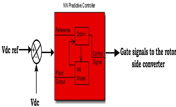
**Fig. 3.** Block diagram of the DC link voltage technique with ANN- Predictive.
