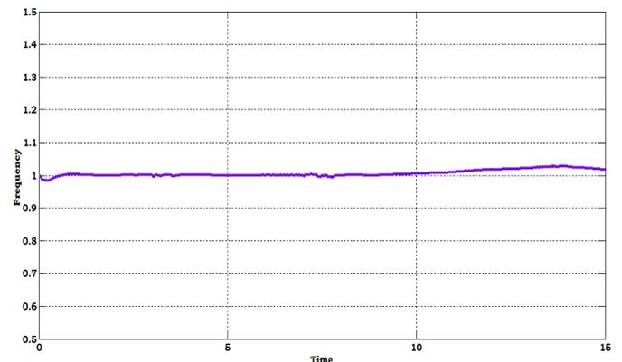
**Fig. 31.** The waveform of frequency of supply when operating system in islanded mode with sudden connection of other units.
