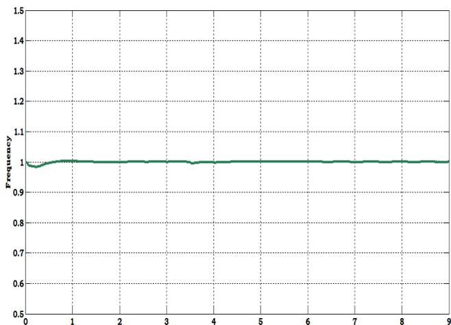
**Fig. 8.** The waveform of frequency of supply when operating system in grid connected mode with sudden disconnection of battery.
