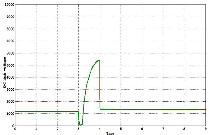
**Fig. 22.** The waveform of DC link voltage across the DC link capacitor when operating system in grid connected mode with sudden disconnection of battery.
