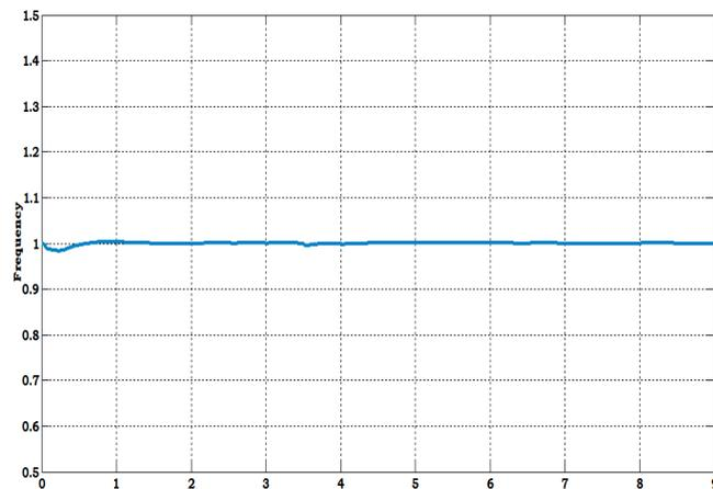
**Fig. 12.** The waveform of frequency of supply when operating system in grid connected mode with sudden fault.
