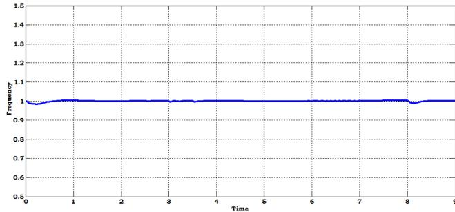
**Fig. 27.** The waveform of frequency of supply when operating system in grid connected mode with sudden fault.
