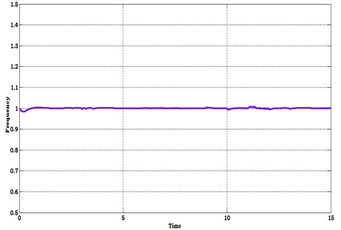
**Fig. 25.** The waveform of frequency of supply when operating system in grid connected mode with sudden connection of other units.
