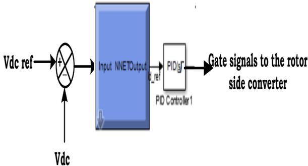
**Fig. 2.** Block diagram of DC- link voltage technique with ANN-PID.
