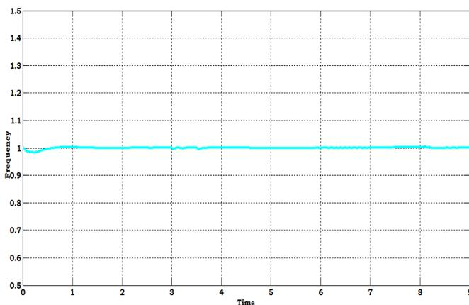
**Fig. 33.** The waveform of frequency of supply when operating system in islanded mode with sudden fault.
