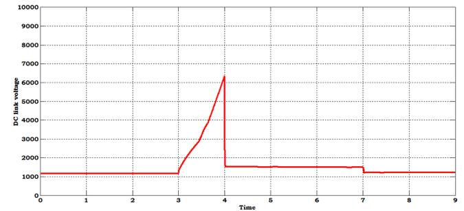
**Fig. 13.** The waveform of DC link voltage across the DC link capacitor when operating system in islanded mode.
