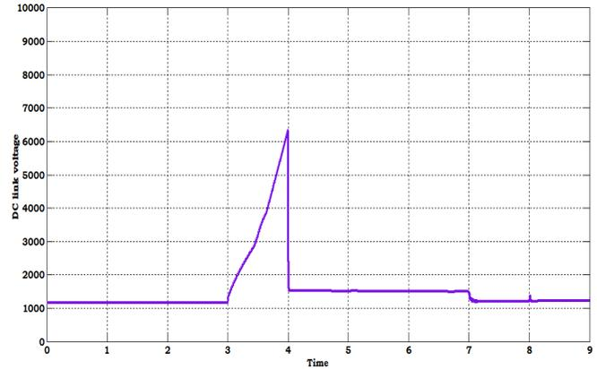
**Fig. 17.** The waveform of DC link voltage across the DC link capacitor when operating system in islanded mode with sudden fault.
