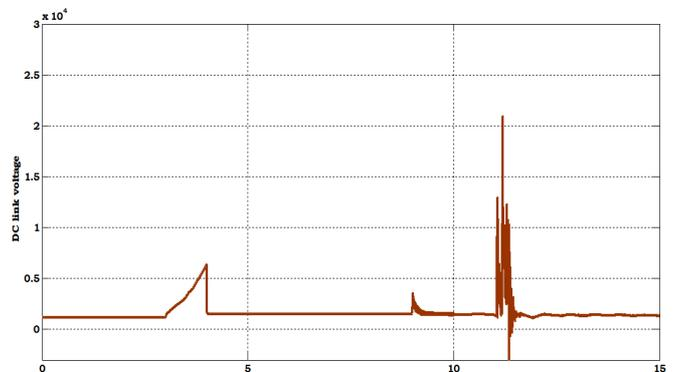
**Fig. 9.** The waveform of DC link voltage across the DC link capacitor when operating system in grid connected mode with sudden connection of other units.
