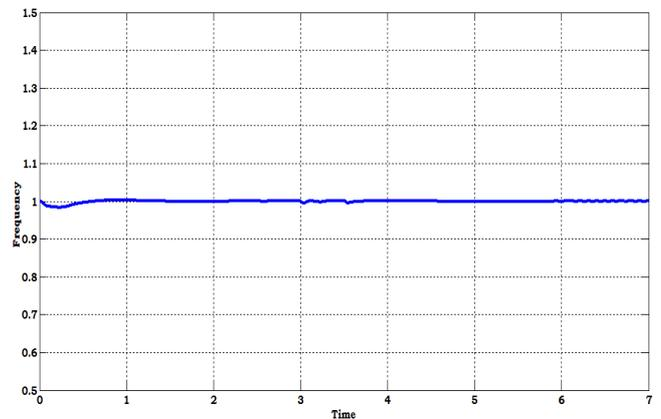
**Fig. 21.** The waveform of frequency of supply when operating system in grid connected mode with battery.
