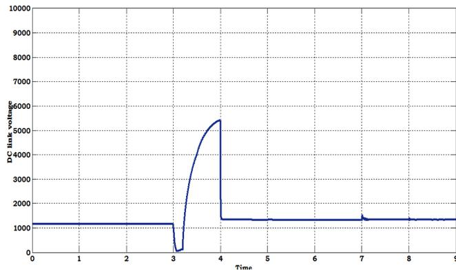
**Fig. 32.** The waveform of DC link voltage across the DC link capacitor when operating system in islanded mode with sudden fault.
