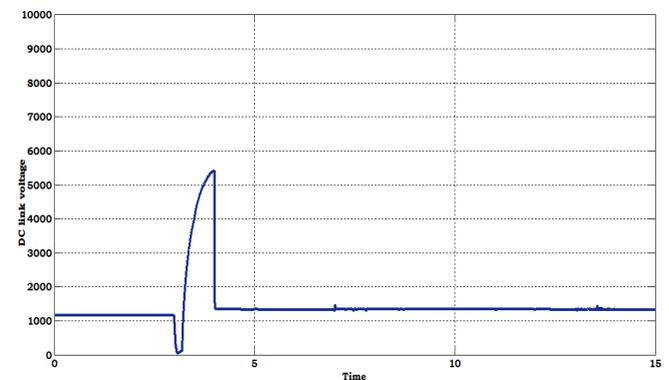
**Fig. 30.** The waveform of DC link voltage across the DC link capacitor when operating system in islanded mode with sudden connection of other units.
