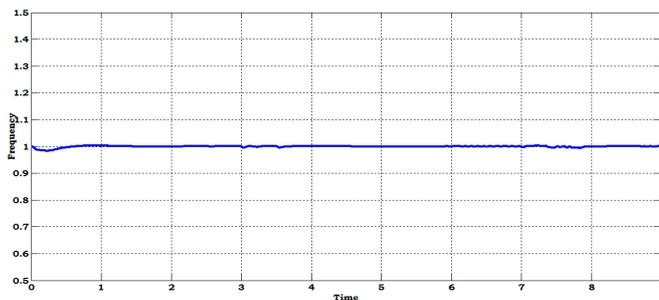
**Fig. 29.** The waveform of frequency of supply when operating system in islanded mode.
