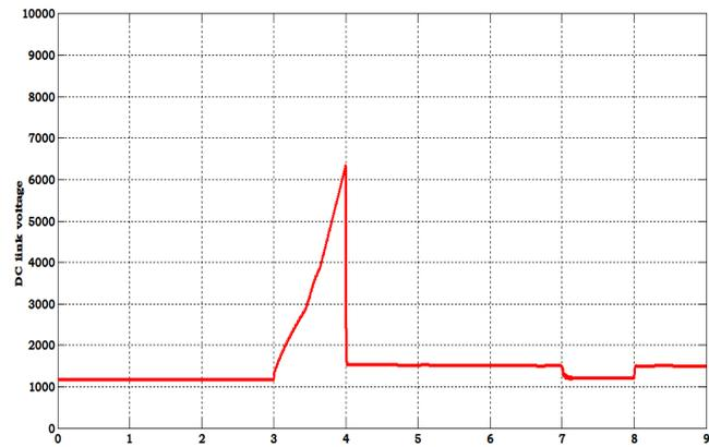
**Fig. 11.** The waveform of DC link voltage across the DC link capacitor when operating system in grid connected mode with sudden fault.
