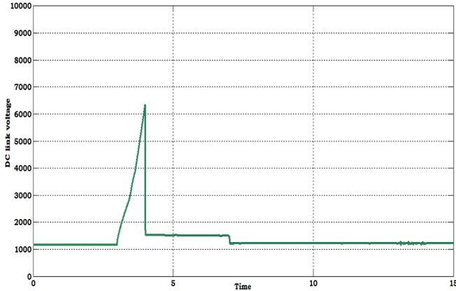
**Fig. 15.** The waveform of DC link voltage across the DC link capacitor when operating system in islanded mode with sudden connection of other units.
