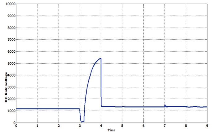
**Fig. 26.** The waveform of DC link voltage across the DC link capacitor when operating system in grid connected mode with sudden fault.
