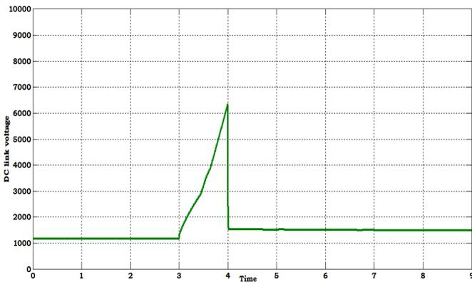
**Fig. 7.** The waveform of DC link voltage across the DC link capacitor when operating system in grid connected mode with sudden disconnection of battery.
