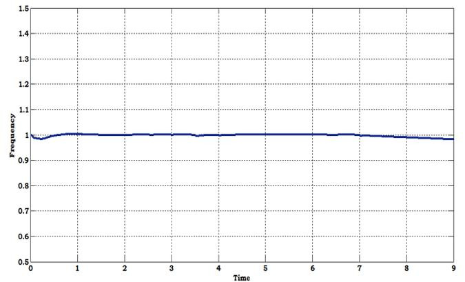
**Fig. 14.** The waveform of frequency of supply when operating system in islanded mode.
