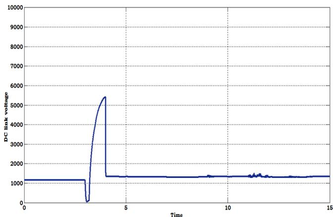
**Fig. 24.** The waveform of DC link voltage across the DC link capacitor when perating system in grid connected mode with sudden connection of other units.
