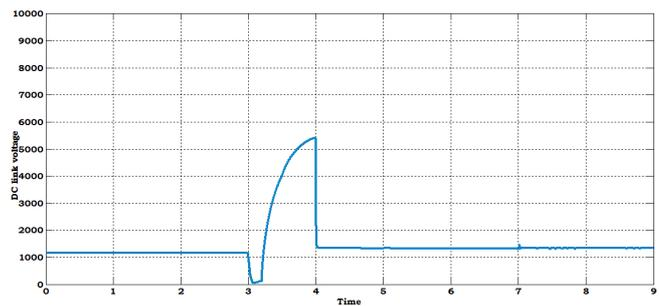
**Fig. 28.** The waveform of DC link voltage across the DC link capacitor when operating system in islanded mode.
