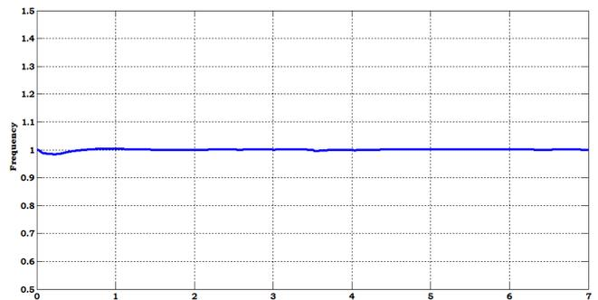
Fig. 6. The waveform of frequency of supply when operating system in grid connected mode with battery.
