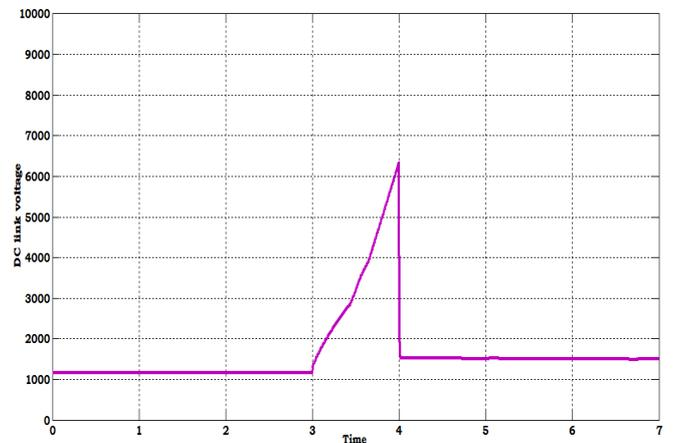
**Fig. 5.** The waveform of DC link voltage across the DC link capacitor when operating system in grid connected mode with battery.
