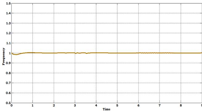
**Fig. 23.** The waveform of frequency of supply when operating system in grid connected mode with sudden disconnection of battery.
