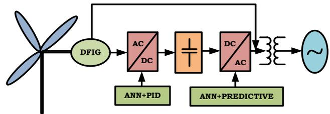
**Fig. 1.** Block diagram of the controlled DFIG based wind turbine.
