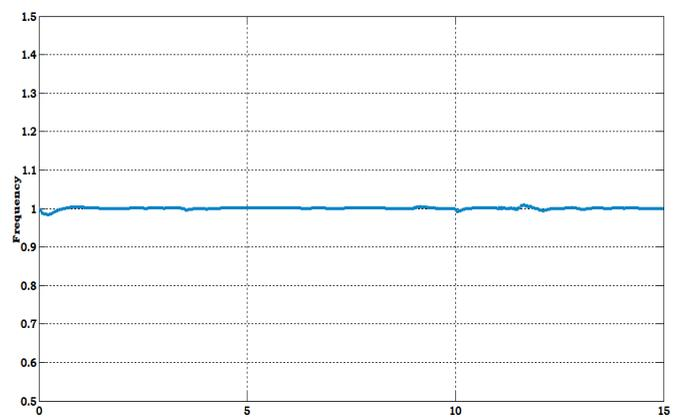
**Fig. 10.** The waveform of frequency of supply when operating system in grid connected mode with sudden connection of other units.
