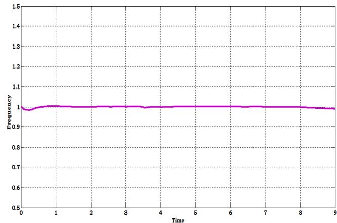
**Fig. 18.** The waveform of frequency of supply when operating system in islanded mode with sudden fault.
