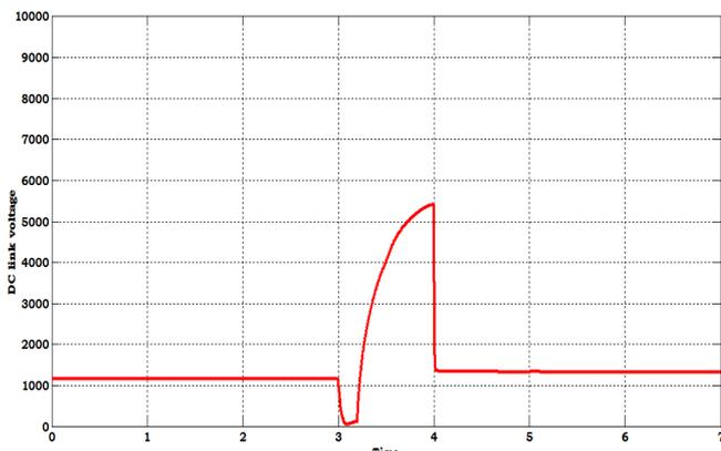
**Fig. 20.** The waveform of DC link voltage across the DC link capacitor when operating system in grid connected mode with battery.
