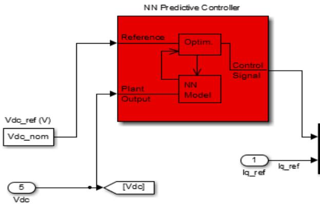
**Fig. 19.** Simulink diagram of NN fed with predictive controller.
