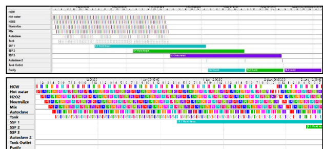
Fig. 2. Gantt chart showing the bioethanol production process from oil palm empty fruit bunches with the SSF 3 tank after adding more cycles to the pretreatment process
