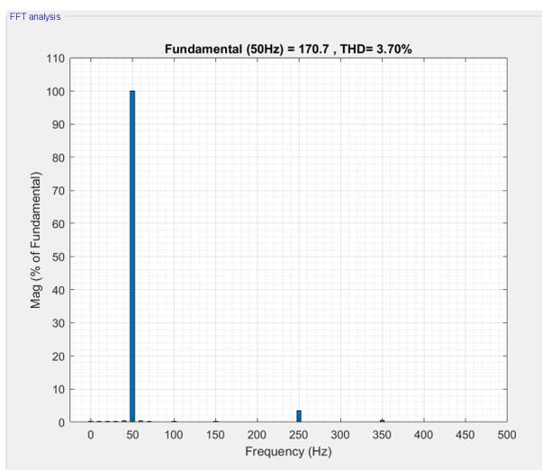
**Fig. 11.** FFT analysis using SBM technique.
