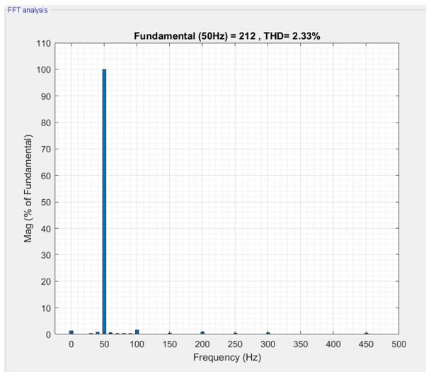
**Fig. 10.** FFT analysis for the employed unipolar PWM.
