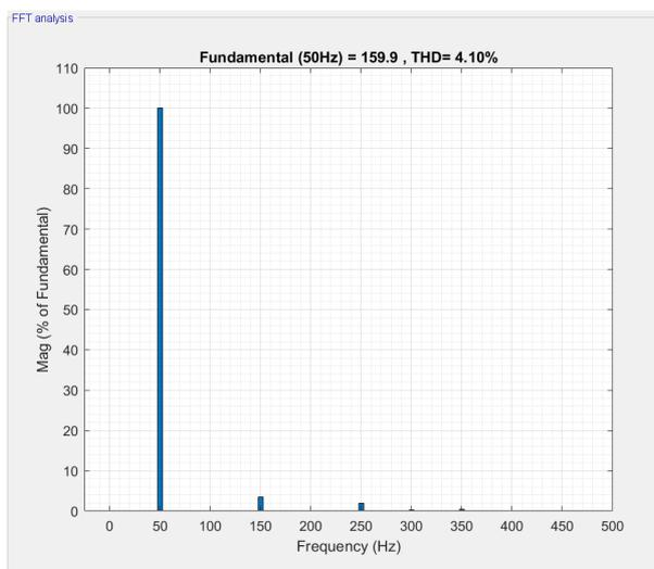
**Fig. 12.** FFT analysis using MBM technique.
