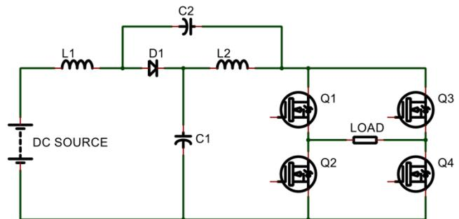
Fig. 2. Voltage fed quasi Z-source inverter.
