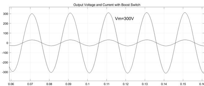
**Fig. 8.** Peak phase voltage-current with boost switch  $Q_5$ .
