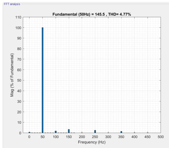
**Fig. 13.** FFT analysis using MCBM technique.
