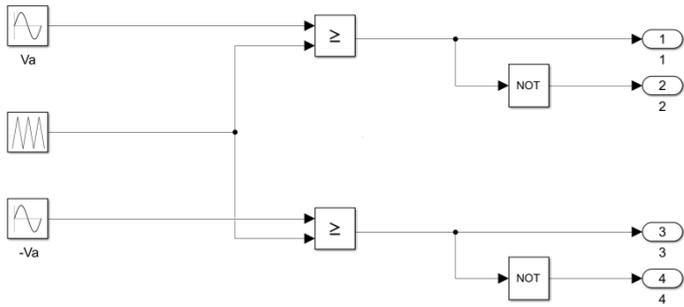
Fig. 3. Unipolar PWM technique block scheme.
