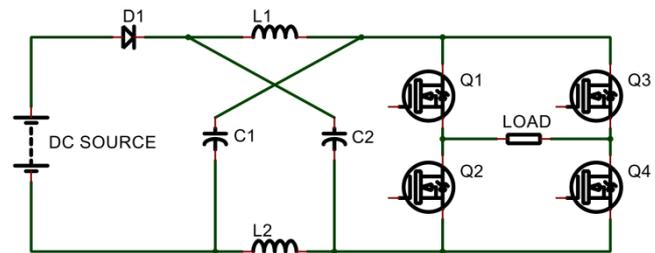
Fig. 1. Voltage fed Z-source inverter.
