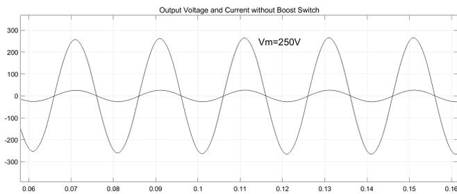
**Fig. 7.** Peak phase voltage-current without boost switch  $Q_5$ .
