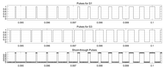
Fig. 6. Generated pulses and the shoot-through pulses.
