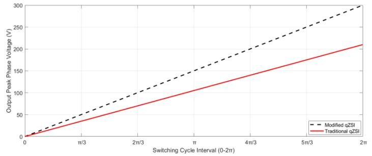
**Fig. 9.** Comparison of the peak phase voltages at  $V_{DC}=100V$ .
