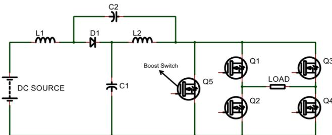
Fig. 5. Modified qZSI circuit with additional boost switch.
