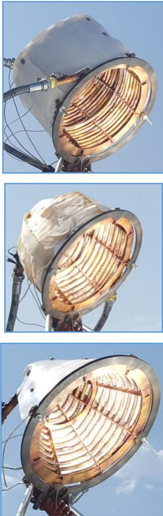
**Fig. 9.** Photographs of the PDC<sub>cr</sub> models after being placed in the focal center of the dish collector
