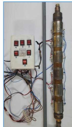
Fig. 3. Photograph of the heating source for the HTF inlet
