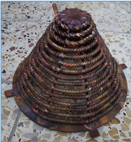
**Fig. 6.** Photographs of the PDC<sub>cr</sub> models after the copper structure was wrapped with the twisted tube
