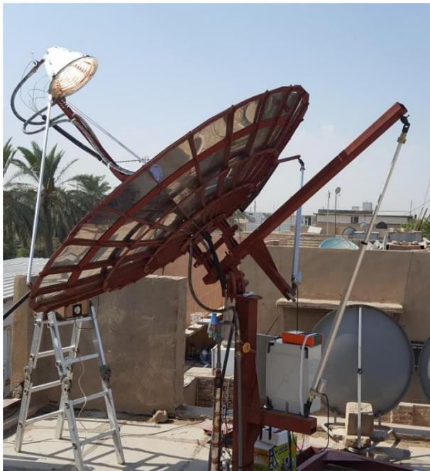
Fig. 1. Photograph of the examined solar dish collector with a cavity receiver
