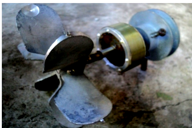
Fig. 5. Impeller, rotor, and pulleys mounted on the blower shaft
