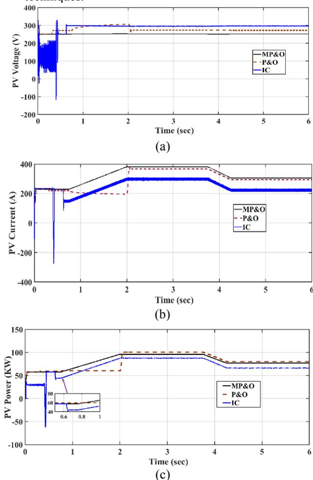
**Fig. 13.** Performance comparison of PV system under ramp change irradiance; (a) output of PV voltage (b) output of PV current, and (c) output of PV power.
