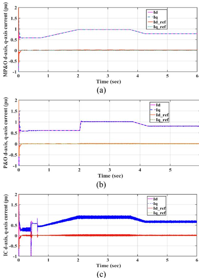
Fig.18. d-axis and q-axis current under different algorithms.
