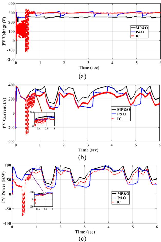
**Fig.20.** Performance analysis comparison of PV system under random change irradiance; (a) PV output voltage (b) PV output current, and (c) PV output power.
