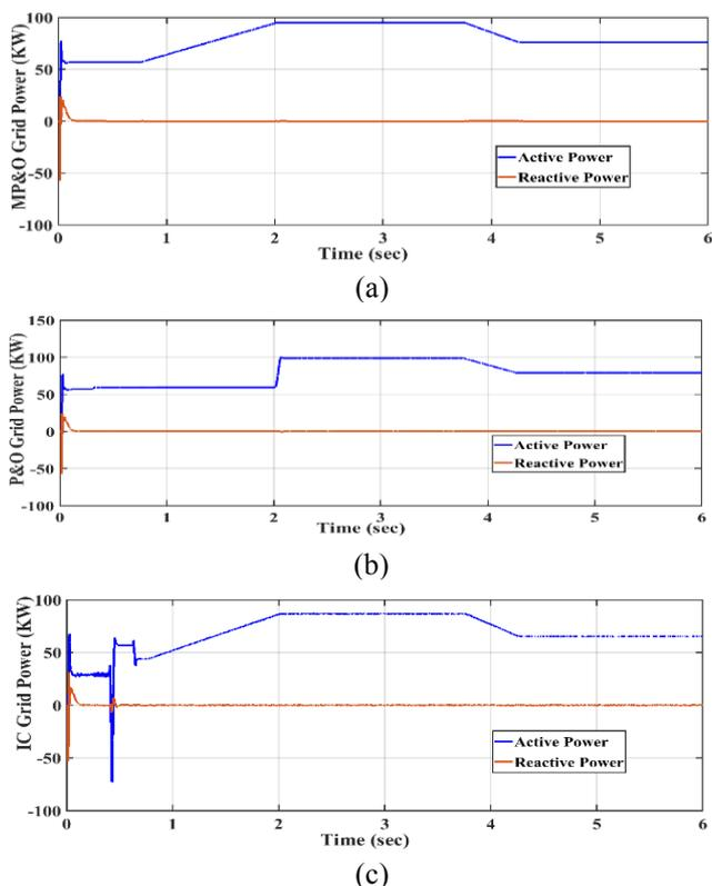
Fig. 17. Grid active and reactive power under different algorithms.
