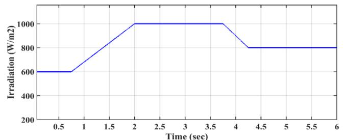
Fig. 12. Irradiance in a ramp changed profile.
