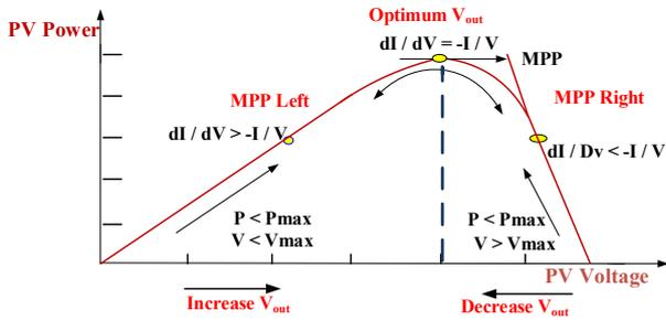
Fig. 6. IC algorithm power - voltage curve.
