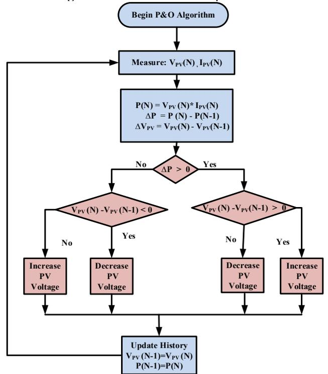
Fig. 9. The P&O algorithm flowchart.
