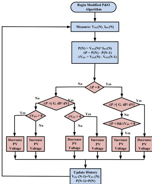
Fig. 11. The MP&O algorithm flowchart.
