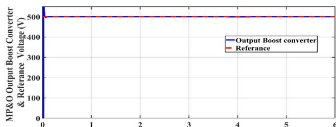
**Fig. 14.** MP&O output boost converter and reference voltage.
