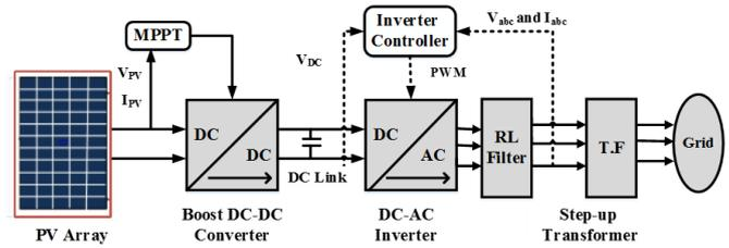
Fig. 1. Simplified diagram of grid connected of PV system.
