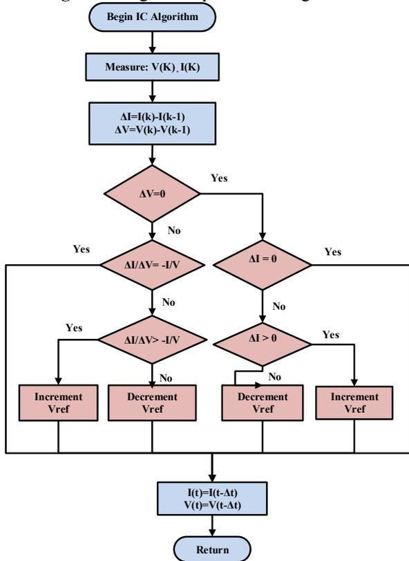
Fig. 7. The IC algorithm flowchart.
