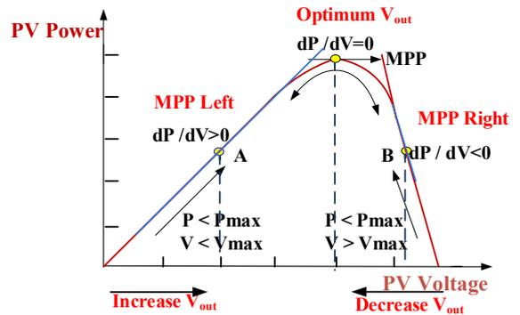
Fig. 8. P&O three modes of operation.
