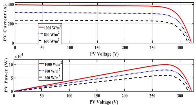
Fig. 3. I-V and P-V characteristics curves under variable irradiation.
