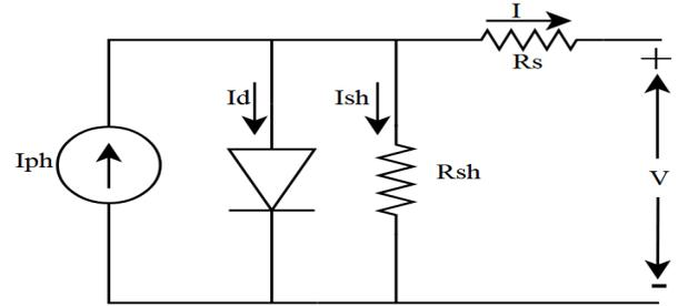
Fig. 2. Single-diode equivalent circuit of a PV cell.
