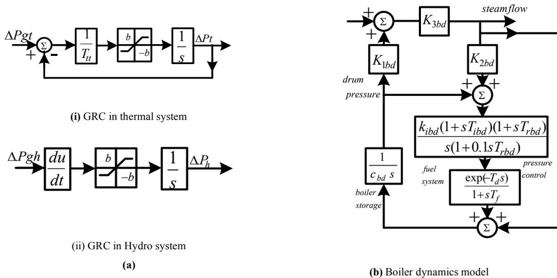
Fig. 2. (a) GRC for thermal, and hydro system, (b) boiler dynamics for thermal system.
