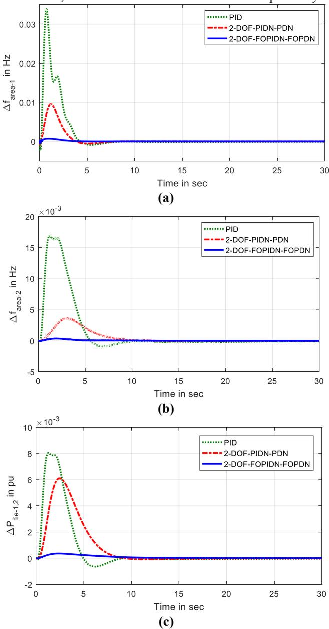
**Fig. 5. (a)** Frequency deviation in area-1, **(b)** frequency deviation in area-2, **(c)** power deviation in the tie-line.
