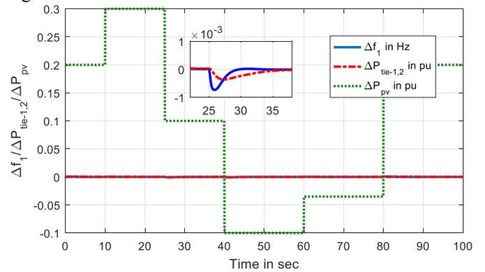
**Fig. 6.** Time diagram of solar power variation, frequency deviation, and tie-line power deviation.
