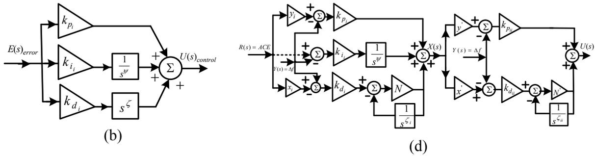
**Fig. 3.** (a) Working co-ordinate of PI, and FOPID controller, (b) structure of FOPID controller, (c) structure of cascade controller, (d) structure of 2-DOF-FOPIDN-FOPDN controller.
