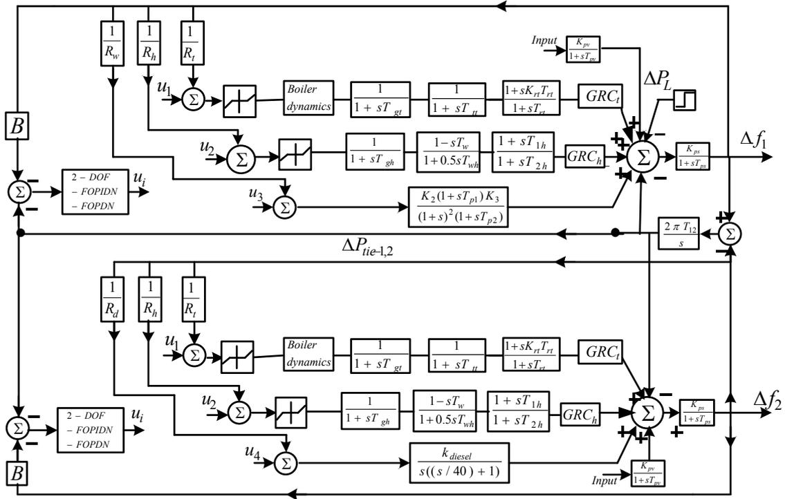
Fig. 1. Model of the two-area power system containing renewable sources.
