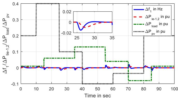
**Fig. 7.** Time diagram of solar power variation load variation, frequency deviation, and tie-line power deviation.
