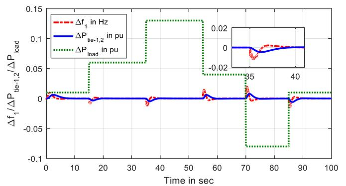
**Fig. 8.** Time diagram of load variation, frequency deviation, and tie-line power deviation.
